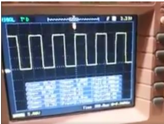
Figure 3 - PWM Output Signal at TP2
