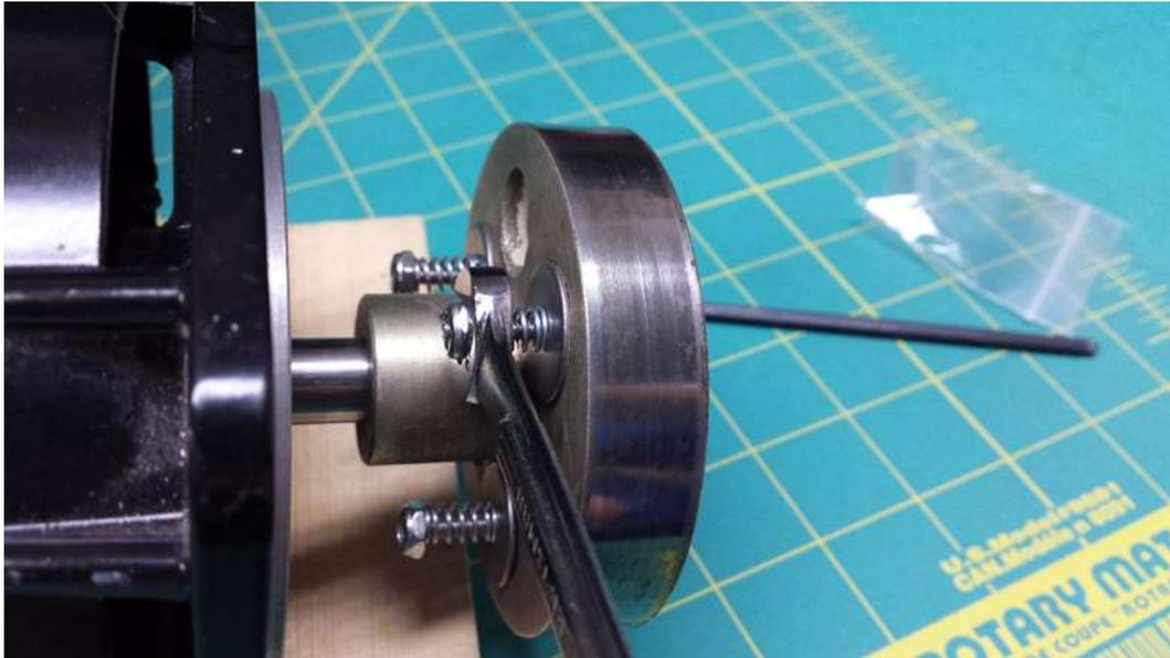
**STEP 10** – The threads should just protrude from the back side of the lock nuts. You may also add some LokTite to the threads if desired. **DO NOT OVER TIGHTEN THE NUTS AND COMPRESS THE SPRINGS TOO TIGHTLY.**
