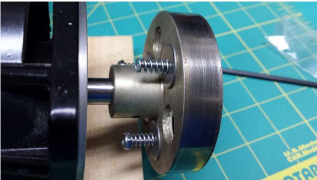
**STEP 9** – Next, tighten the lock nuts with a wrench till the threads just exit the back side of the nylon lock washer. Do not over tighten the screws, the nylon thread locks will hold the screws firmly in place.
