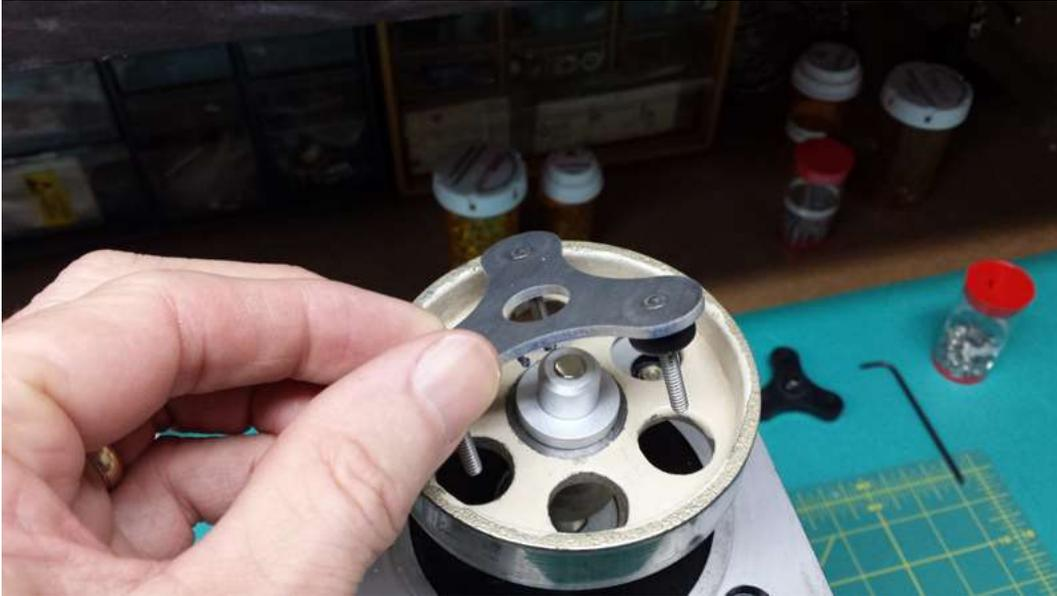
**STEP 6** – The spanner should rest on the magnet spindle face and serves as a clamp to hold the spindle firmly. Hold the spanner in place by hand while laying the motor back over on its side.
