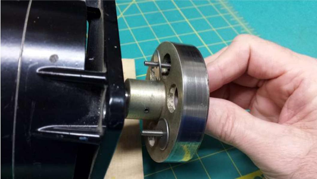
**STEP 8** – Add a spring to each of the threaded studs on the back sides of the washers and finger tighten the lock nuts just enough to hold the assembly in place.
