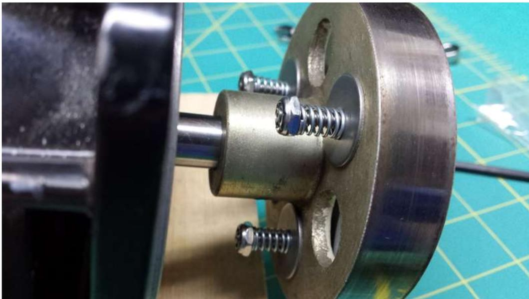
**STEP 11** – Inspect the spanner and magnet spindle to make sure it's held firmly in place. Align the spanner so the threads and washers are centered in hole. It should be tight enough you can move it by hand, but not loose such that it could move from motion of the motor. You may tighten the nuts a little if more pressure is desired, but do not over tighten to avoid bending the aluminum spanner plate.
