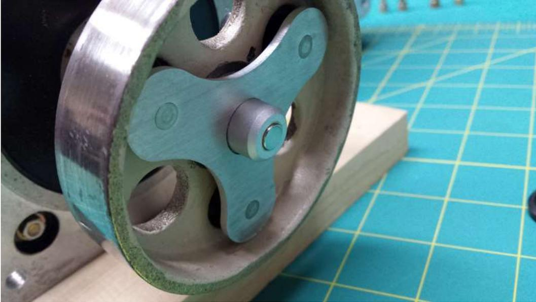
**STEP 12** – Hold the brake solenoid mechanism on the motor to release the brake and spin the motor brake hub by hand. The magnet must spin true without wobble or excessive run out.
