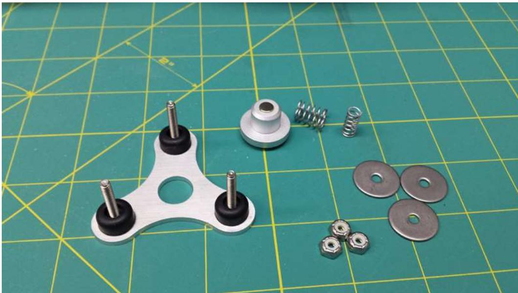
**STEP 3** – The magnet spindle is held into the brake hub so it sits flush against the brake hub face. The ½” center boss on the back side of the magnet spindle should fit snugly into the end of the brake hub with the body of the spindle sitting flush against the brake up face.
