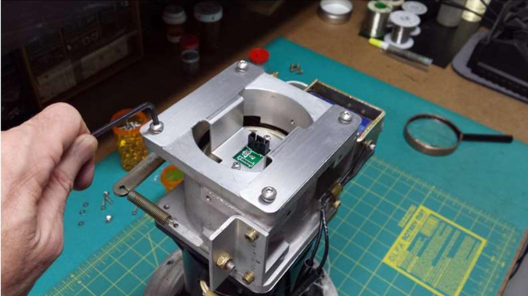
**STEP 16** – Next connect one end of the encoder cable to the encoder and secure the cable to the motor housing with a tie strap. Note the cables are marked TAKEUP and SUPPLY and should be installed on the correct motor for each. The motors are now ready to be installed back into the machine.
