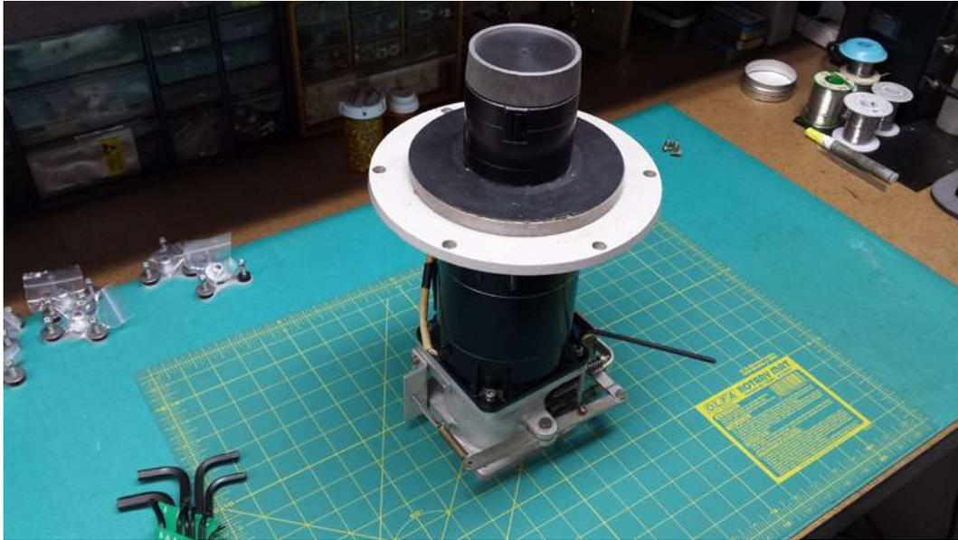
**STEP 2** – Locate the magnet spindle, spanner bracket, springs washers and lock nuts from the kit.
