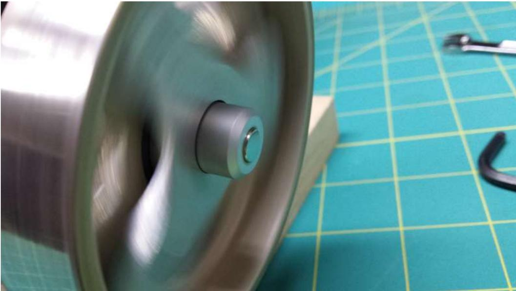
**STEP 13** – Reinstall the brake hub housing and secure the Allen screws holding the brake housing.
