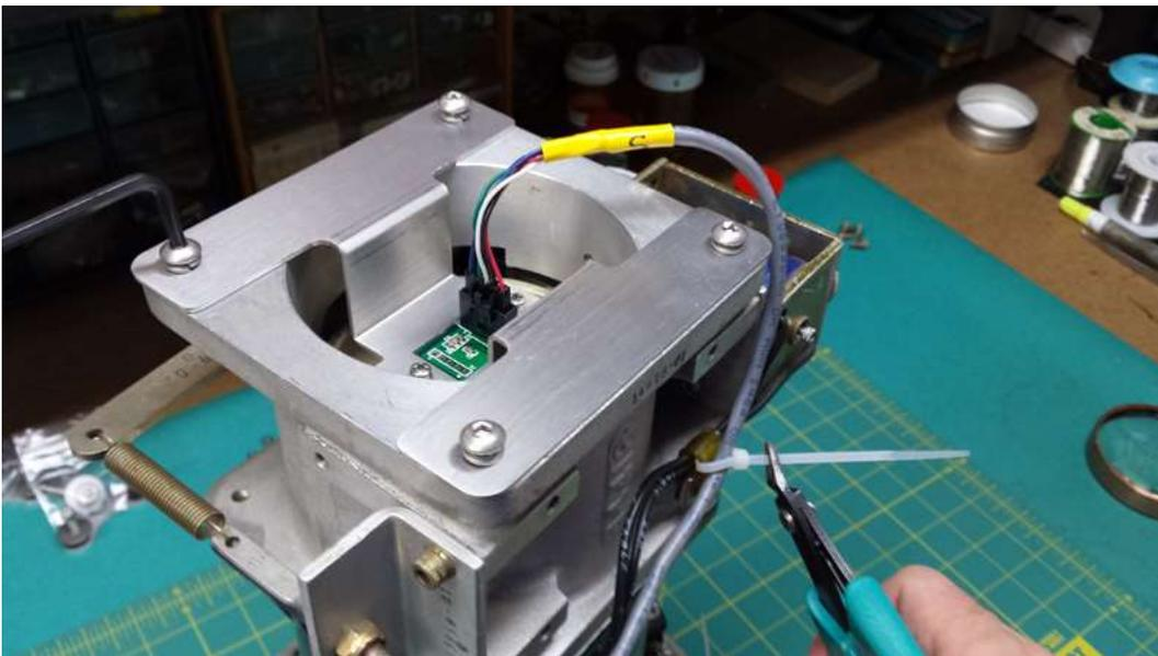
**STEP 17** – Route the cables from the motor quadrature encoders through the machine to the front side of the transport control card cage when installing the motors. Note the TAKEUP and SUPPLY reel encoders must be plugged into the correct connectors as labeled on the DTC-1200 board. Make sure the TAKEUP encoder cable connector is plugged into the TAKEUP encoder connector J3. Likewise, the SUPPLY encoder should be plugged into the SUPPLY connector J2 on the DTC-1200 board.
