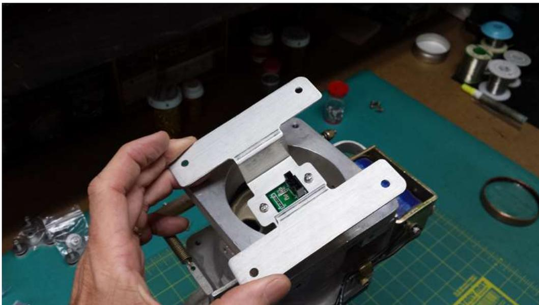
**STEP 15** – Secure the encoder bracket with the lock washers and Allen screws provided. The screws should be tightened snug, but do not over tighten.
