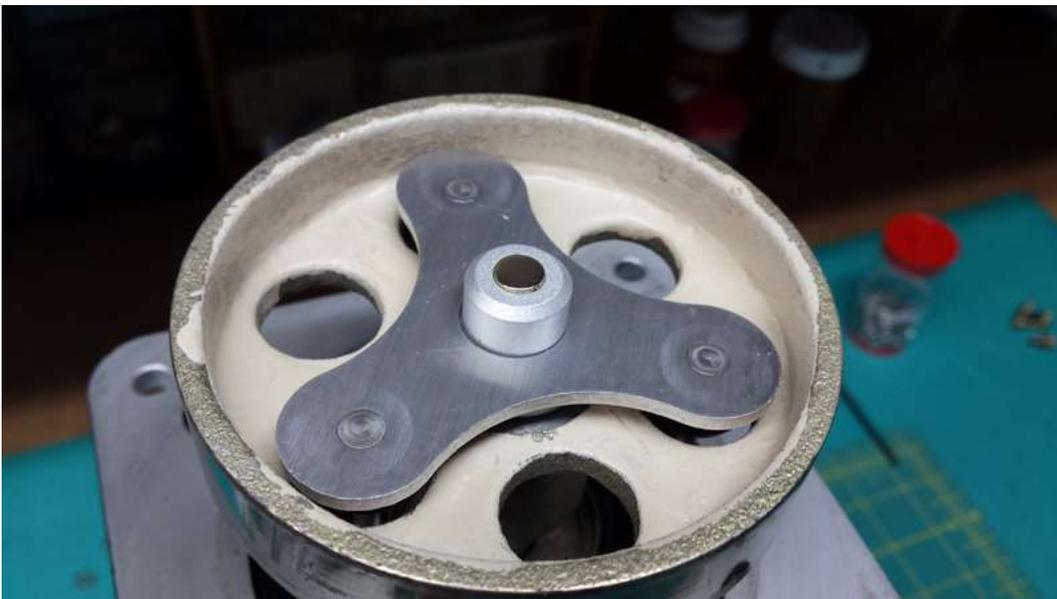
**STEP 7** – Add the large diameter washers on the back side of the brake hub while holding the spindle and spanner in place by hand.
