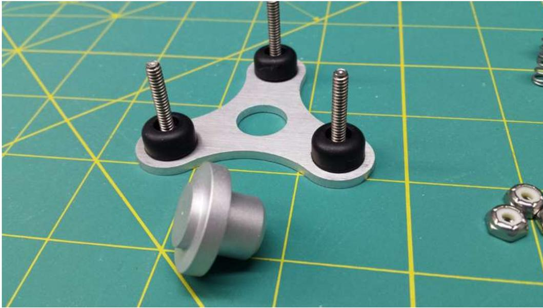
**STEP 4** – Insert the magnet spindle boss end into the brake hub. The boss should fit snug in the hole. If the fit is too tight, use some 400-grit silicon carbide sand paper to smooth the hole in the brake hub.
