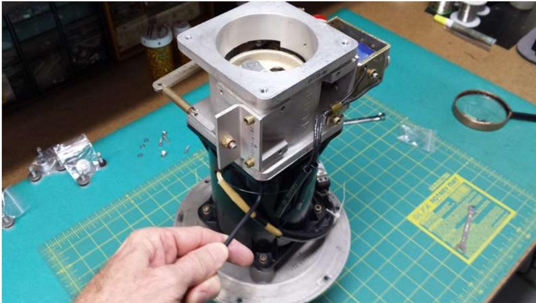
**STEP 14** – Now add the magnetic quadrature encoder assembly on the back side of the brake housing.
